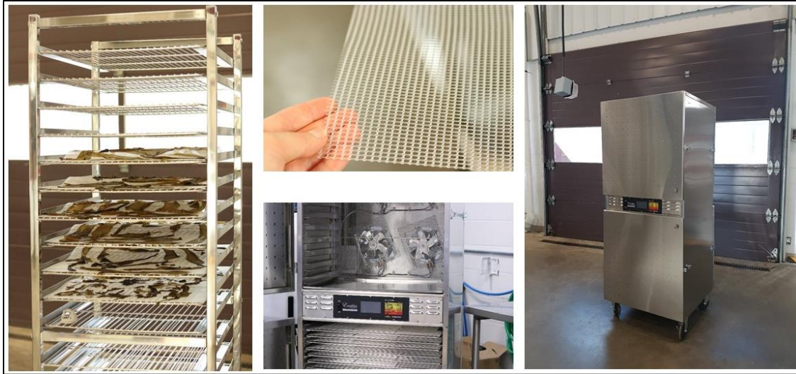
Figure 2. Left: air-dried kelp on a rack-and-roll shelf. Middle top: a plastic tray liner. Middle bottom: Upper and lower chambers of the dehydrator are open (only the lower chamber is loaded with trays). Right: Excalibur COMM2 commercial dehydrator.
