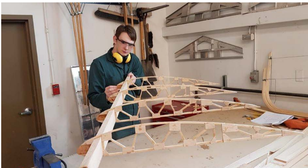
Aircraft Structures Program - Student is building a short take-home wood structure wing assembly.
