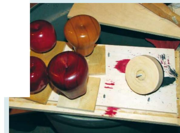
This is the jig which I recently constructed to help me turn a bowl of fruit. It helps me to finish the tops and bottoms of the pieces
